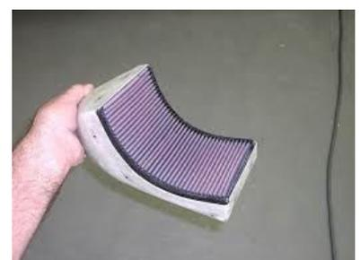
Anyway, here's a trial assembly of the box, with filter. Filter media area is roughly 2X more than a Vans snorkel filter.
