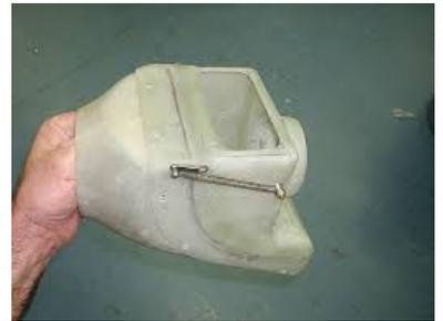
Finished product - process was the usual; epoxy/micro to fill then 80 grit sanding, shell w/epoxy for scratches/pinholes then 180 grit sanding. Primer and two-part single stage color seems to cover 180 grit sanding ok. The exterior cowl surface got primer and K36 sanded to 400 grit as it will later get a two-part pearl topcoat.
